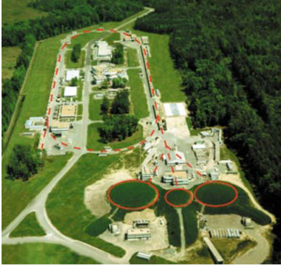
Figure 2.1: Aerial view of Jefferson Lab, where in dashed red depicts the beam line and the red circles represent the locations of the experimental halls. Figure taken from [26].
